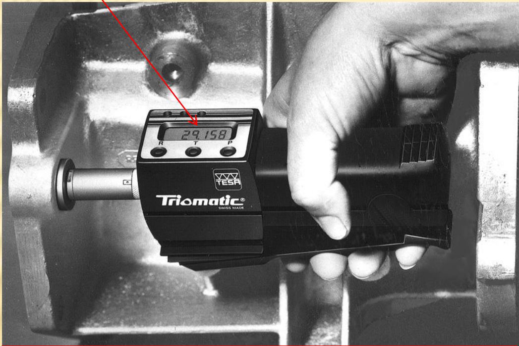
An electronic gage for measuring bore diameters. The measuring head is equipped with three carbide-tipped steel pins for wear resistance. The LED display reads 29.158 mm. Courtesy of TESA SA.
